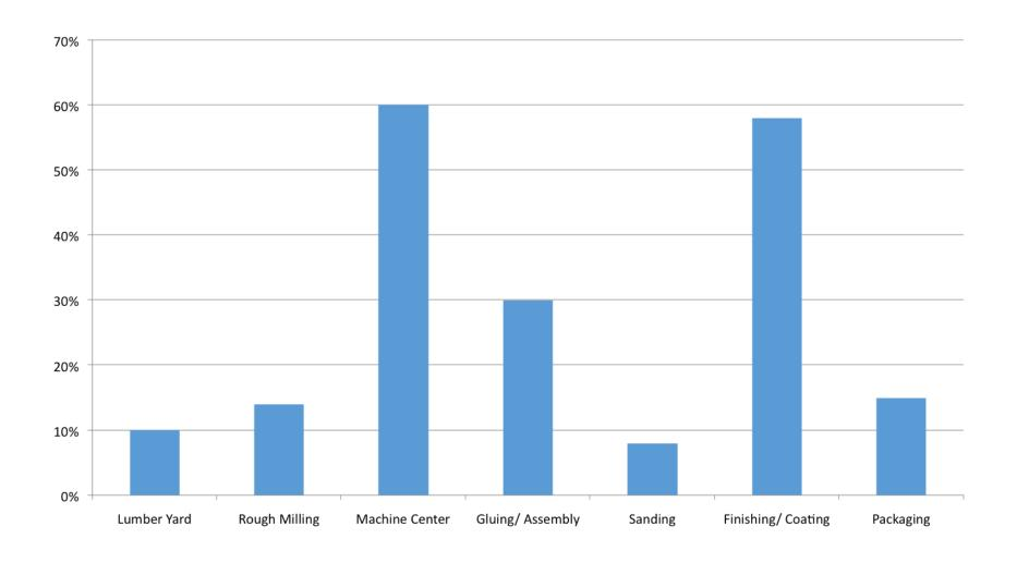
Figure 5. Application of automation in the various stages of furniture manufacturing
