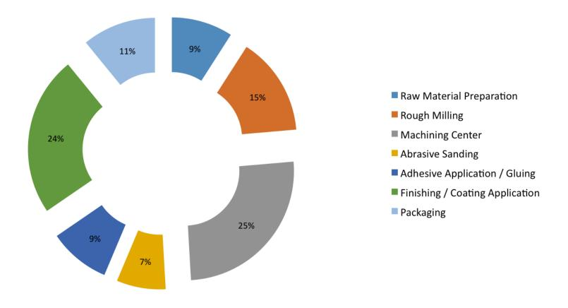
Figure 4. Application of automated technologies in the manufacturing processes of furniture
